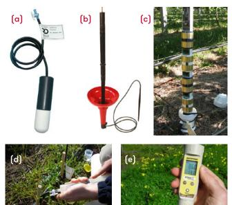
Figure 3: Examples of (a) a suction cup sampler, (b) a wetting front detector, and (c) a capacitance sensor. (d) Extracting soil water samples with a syringe, (e) testing a water sample with a handheld salinity meter. (Photos: SARDI, CSIRO & Sentek Technologies)
