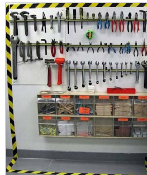
FIGURE 17: STANDARDISED SHADOW BOARD FOR TOOLS
