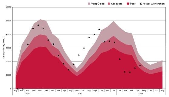
Figure 1: Solar PV performance over 23 months. The shaded areas indicate performance zones. Very good: 90–115 per cent; adequate: 70–90 per cent; poor: 0–70 per cent of rated performance.
