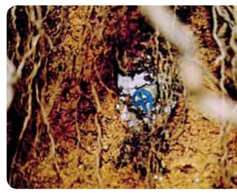
PHOTO 8: GYPSUM BLOCK POSITIONED WITHIN THE ROOTZONE
